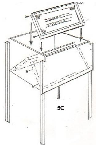
5. Fabricate 2 inner screen frames from 1" x 2" pine, attach with (4) 15/8" deck screws through short 18" side. Attach screening but leave 2 screws loose to allow for adjustment of opening for flies. This should be adjusted after insertion into box body. Refer to drawing 5C & 5D.
