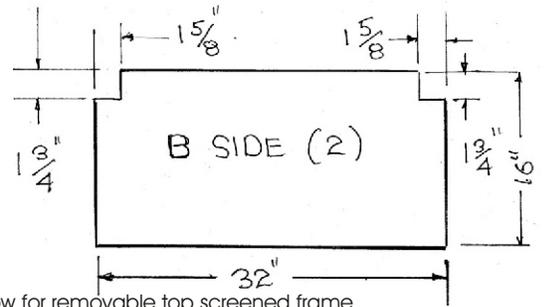
2. Notch upper corners of two sides to allow for removable top screened frame
