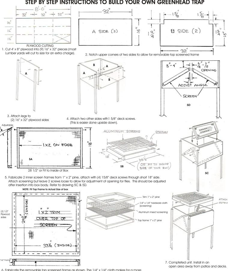
6. Fabricate the removable top screened frame as shown. The 1/4" x 1/4" cloth makes for a more vandal proof unit and is optional. Attach to box with 2 screws. This cover is removed to empty dead flies, service unit and replace Octenal lures. Attach Octenal lures to inside of box.
