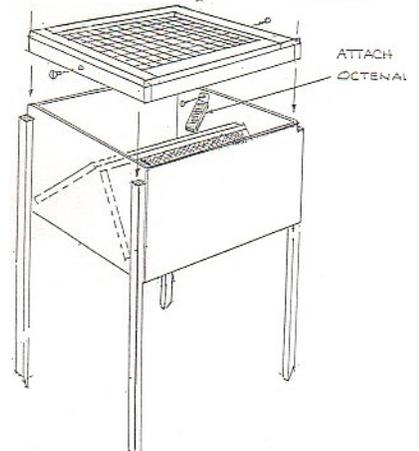
6. Fabricate the removable top screened frame as shown. The 1/4" x 1/4" cloth makes for a more vandal proof unit and is optional. Attach to box with 2 screws. This cover is removed to empty dead flies, service unit and replace Octenal lures. **Attach Octenal lures to inside of box.**
